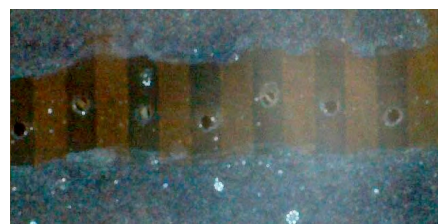
Zoom 400x Dirty Printhead, Before Cleaning Process
